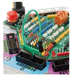
2. Repeat step 1 for the 3V and 5V pins of the TOP which should connect to the 3 and 5 pins of port D respectively.
