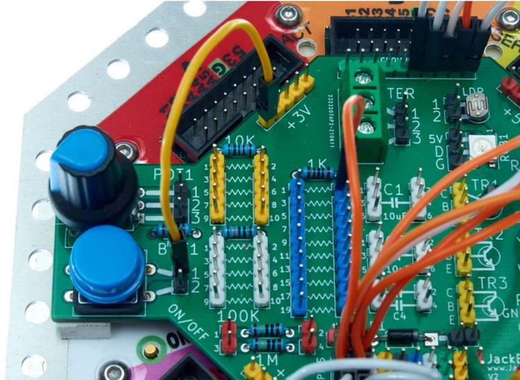
The button is the round blue circle on the lower left and the yellow jumper is connected to pin 1.
