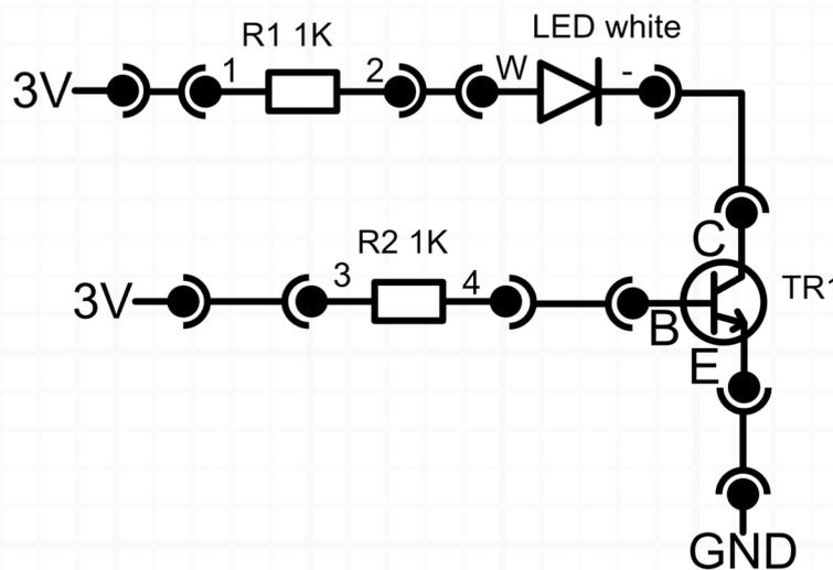
In the circuit the transistor is TR1 and is used to supply power to the LED when the transistor is turned on. To turn it on we apply 3V to the transistors base as shown above.
