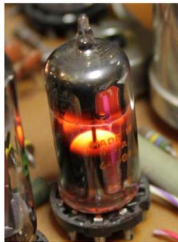
The heat generated by these valves made their use in computers, as switches, very problematic because they would fail after a short time. One of the original valve computers called ENIAC, built in 1946, used 17,468 valves, 70,000 resistors, 10,000 capacitors, 1,500 relays and 6,000 manual switches. It weighed 27 tons, occupied 1,500 square feet of floor space and used 150,000W of electricity.
