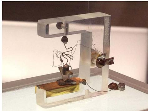
As mentioned above valves are made from glass and thus fragile, they are also very big and consume a lot of electricity. Transistors by comparison are small, robust and consume very little power. And almost as importantly they could switch a lot faster than even the best valves.
