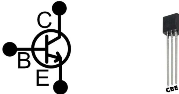
The pins are also shown on a transistor on the right that is the same as the ones on the TOP. The pins are:
