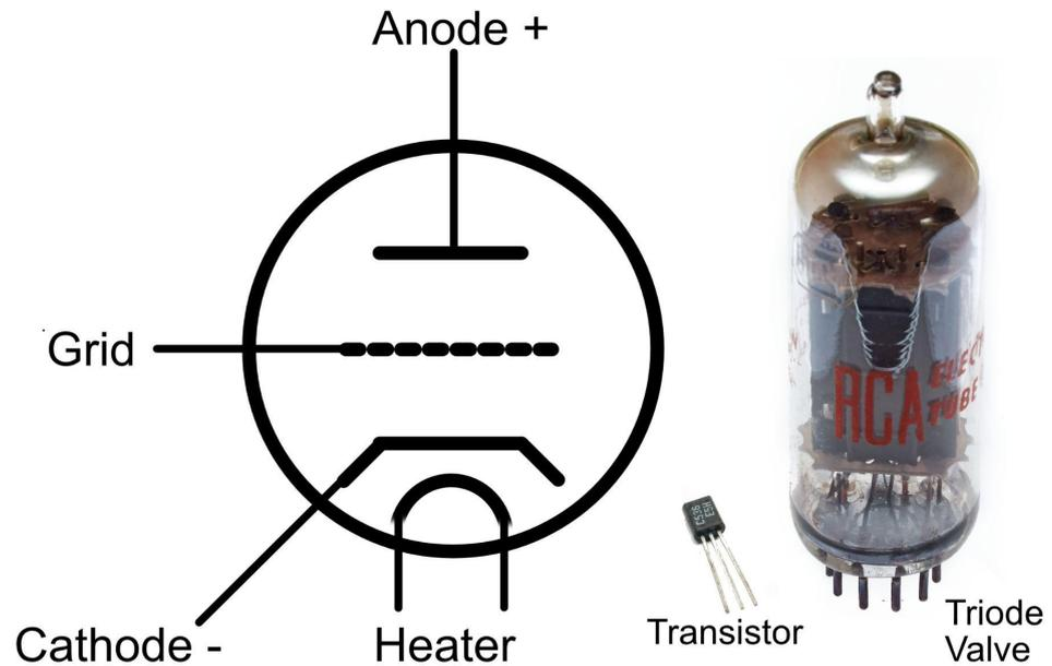
The inside of a valve is shown on the left. First we have the Anode, at the top, which is connected to the positive power supply. Below that we have the Grid which is used to control the amount of current that can flow between the Anode and the Cathode. The Cathode connects to the negative power supply.
