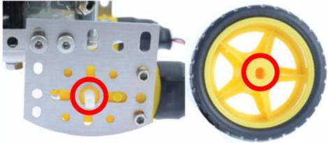
You'll notice that both the wheel and the shaft have a rectangular shape, so make sure that they are lined up before you push the motor on. You'll know the motor is on securely when it clicks.
