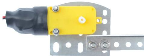
3. Now, do the same for the right motor. Line up the two right-most holes on the inside of the right angle plate with the two left-most holes on the inside of the motor's plate. Attach with two bolts, inserting from the outside and attaching washers and nuts from the inside.
